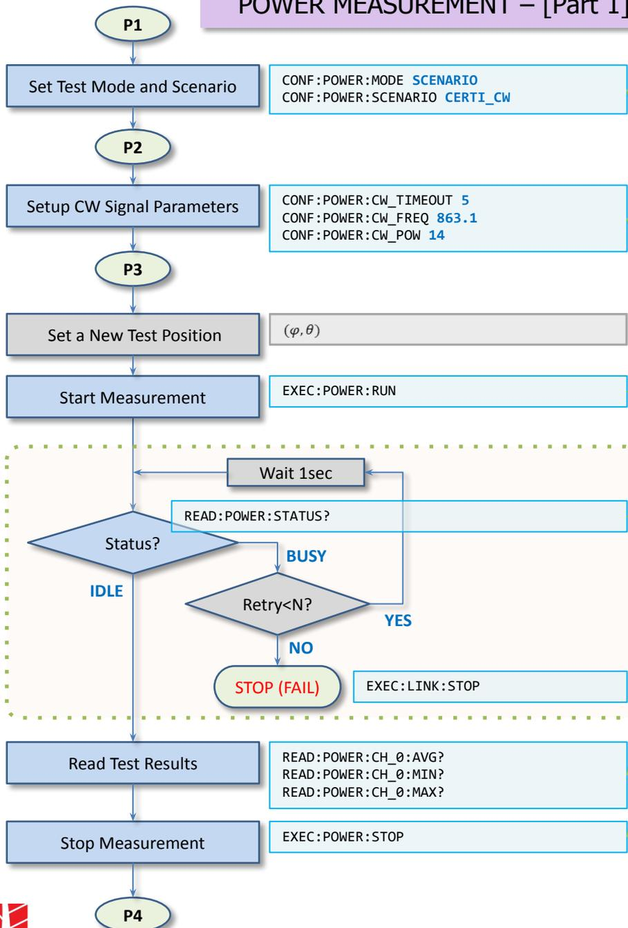
We propose two different methods in implementing measurement of 3D pattern of TX power;
